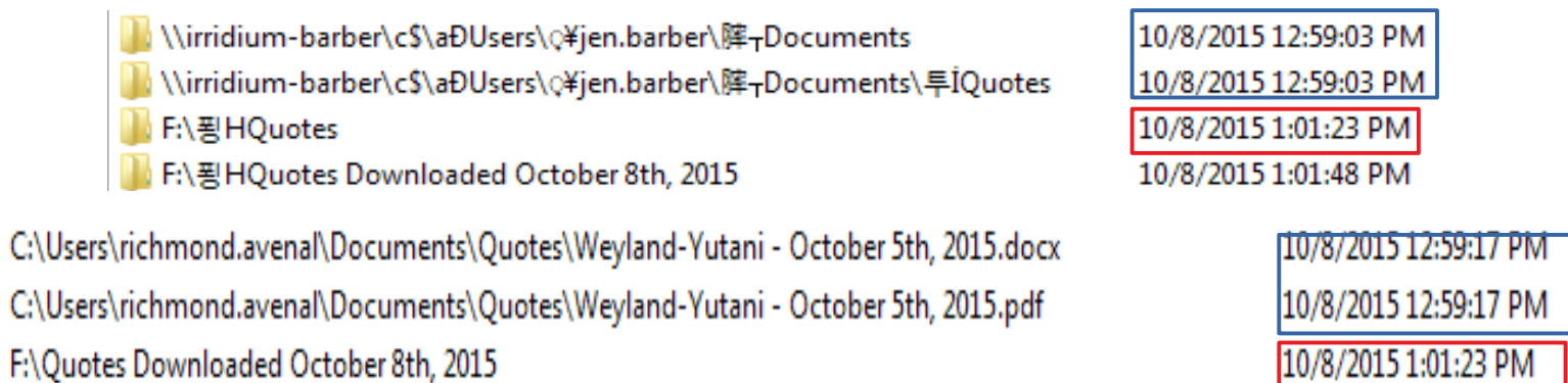
Figure 4. A comparison of shellbags (top) versus jump lists (bottom) recovered early 10/8/2015. PC accesses Jen Barber’s documents through the network folder at 1:59 PM (local time), and new files appear in Richmond’s document at 1:59:17. A USB device is accessed at 2:01 PM
